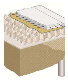
GeoVoid design for each application is determined based upon the thickness (t) and depth (d) of the GeoVoid compressible fill material.
